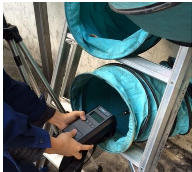
Fig. 1 Measurement by particle counter
